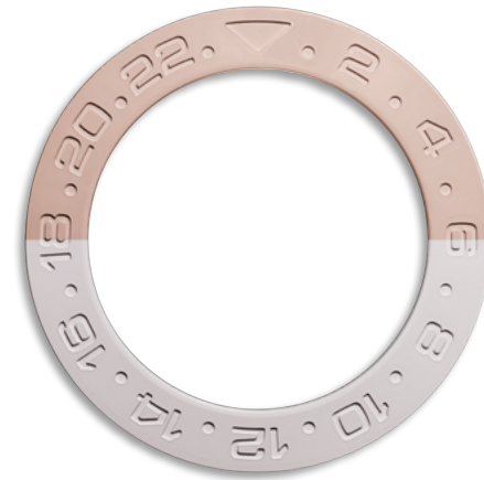
Insert after impregnation with aqueous solution
